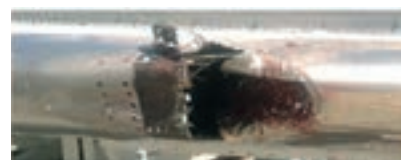
(fig.7) Damage to horizontal tail plane after bird strike test
